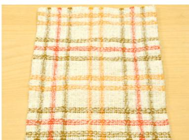
Fig. 3 Electric conductive fabric. (CS6001, Shibata Technotex) [3]
