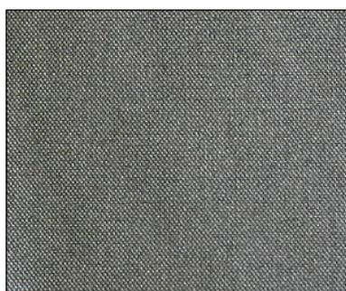
Fig. 2 Electric conductive fabric. (Osaka Electronics Industry)
